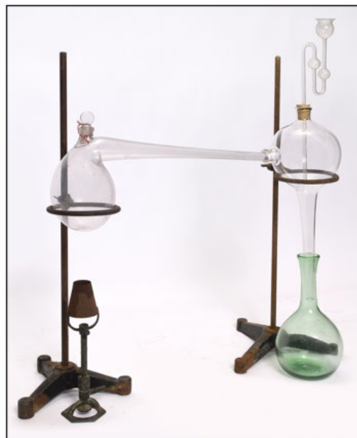
Figure 13. Large retort with an alternative orientation for a quilled receiver fitted with a safety tube.
