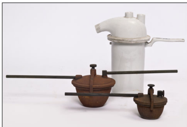
Figure 8. Examples of iron and porcelain laboratory-scale retorts. The detachable beak of the porcelain retort is missing.
