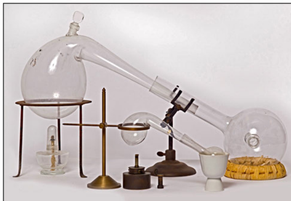
Figure 9. Range of glass retort sizes found in the Jensen-Thomas Apparatus Collection illustrated using a 1.5 L, c. 1860, lime-glass, tubulated retort and tubulated receiver and a 25 mL, c. 1900, soft glass, plain retort with a plain receiver.
