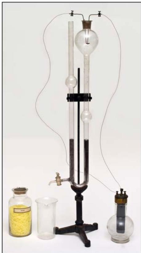
Figure 10. A later example of a Hofmann eudiometer from the Jensen-Thomas Apparatus Collection used for demonstrating volume changes in solid-gas reactions. The glass stopper at the top of the bulb is missing.
