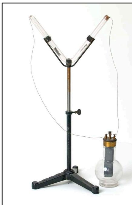
Figure 5. A later version of the Hofmann V-cell for electrolysis from the Jensen-Thomas Apparatus Collection. It is being powered by a Grenet dichromate cell.
