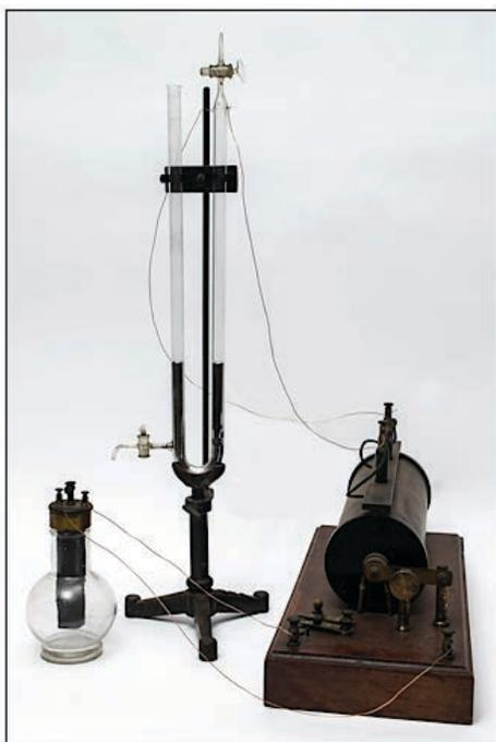
Figure 8. A later version of a Hofmann eudiometer from the Jensen-Thomas Apparatus Collection used for demonstrating the volume changes in gas-gas reactions.
