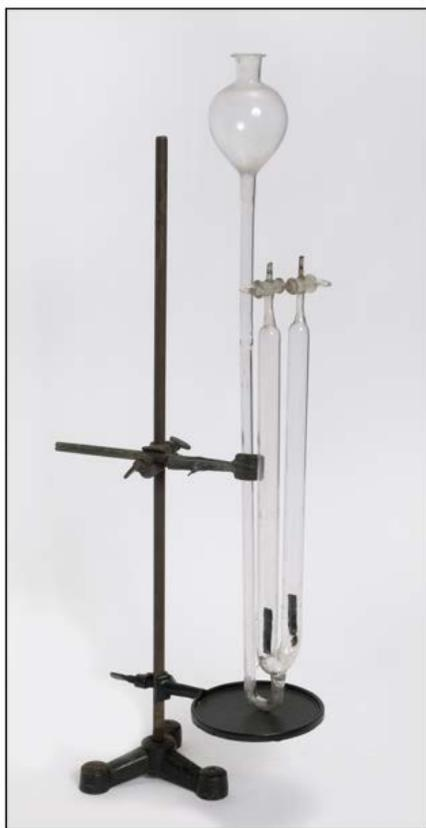
Figure 7. A later version of the Hofmann U-cell for electrolysis from the Jensen-Thomas Apparatus Collection based on his final design of 1869.
