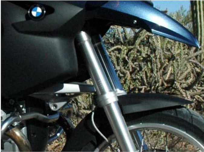
The Saxon-Motodd has an additional swing arm that mounts to the frame and supports the spring. This causes the trail and rake to increase during braking instead of decreasing as with traditional telescopic forks.
