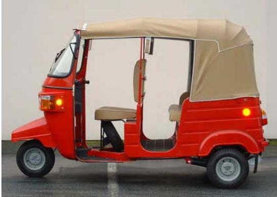
This is a very simple design that has the wheel axle in front of the pivot point and shock. Also, the front wheel is bolted onto the front end, without an axle, which makes maintenance much easier.
