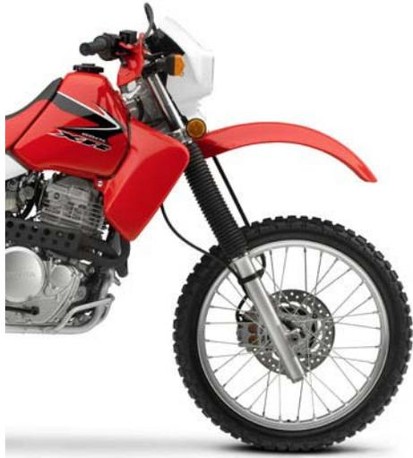
This type of front end is widely used by every motorcycle manufacturer. A fork tube holds a spring and damper, which are resting in oil. The forks can be adjusted for any type of use or performance.
