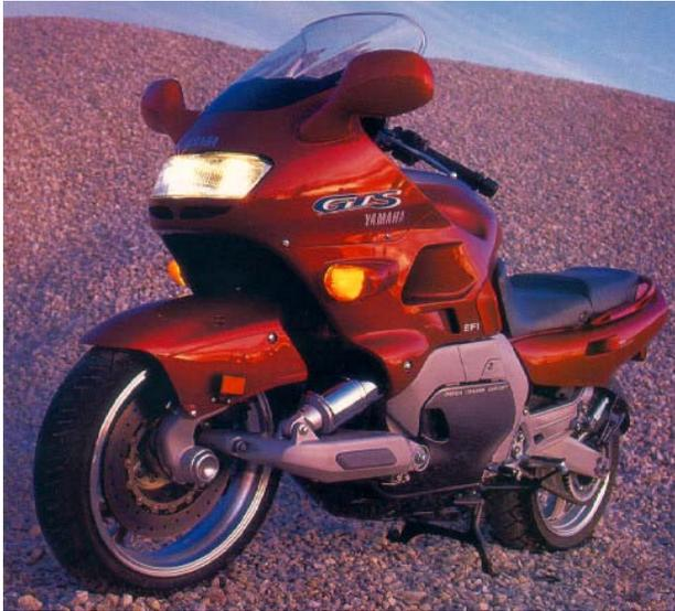
The Rationally Advanced Design (RADD) is very similar to the suspension used on many cars. It is simply a swing arm mounted on the front of the motorcycle to control the front suspension. While a series of spindles and ball joints are used to control the steering of the front wheel.
