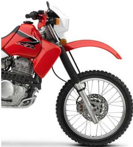
**Figure 6-Internal Spring Design On A Honda XR650**
