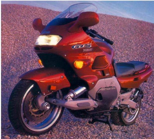
**Figure 2- RADD Design On A Yamaha GTS-1000**
