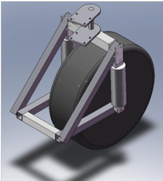
**Figure 7- Front Suspension**
