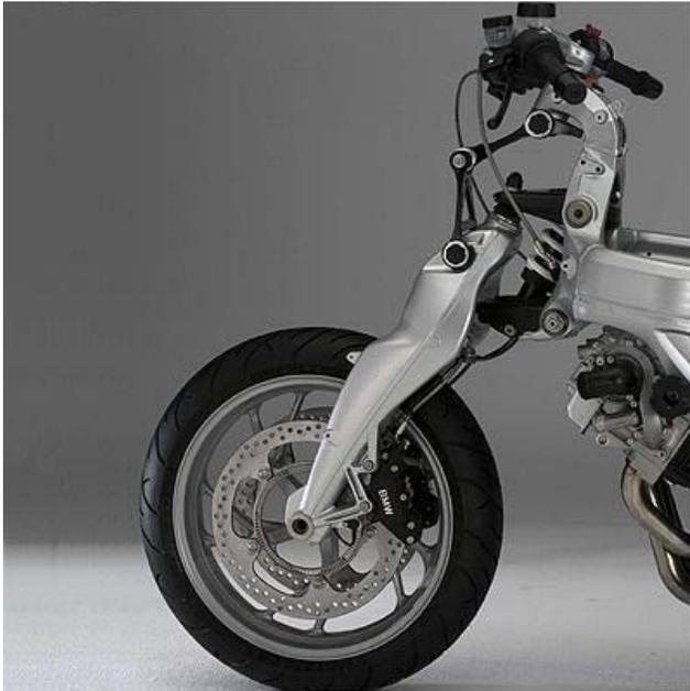
This is a very elegant set up that separates the steering forces from the suspension forces. There are a set of parallel A arms that connect to the front end to handle suspension while a folding linkage controls the steering. While the suspension goes over potholes the geometry of the front end never changes.
