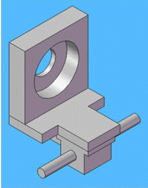
**Figure 8-Rear Suspension Mount**
