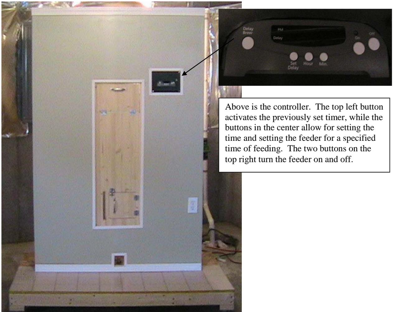
Figure 9 – Completed Prototype (Front)
