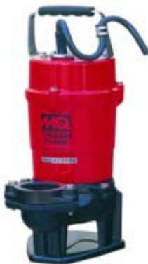
2", 83 GPM, 1/2 HP, 115V, Contractor grade submersible trash pump. Cast iron pump casing for the demanding environments encountered with heavily debris-laden water. Equipped with a 2" discharge port that can easily handle solids up to 1 inch in diameter. A vortex action discharges solids away from the multi-vane impeller. \*\*\* [click here for more detailed info](#) \*\*\*
