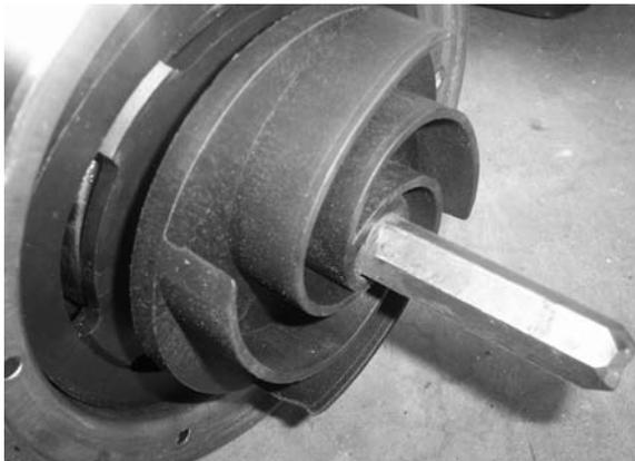
Figure 7: Impeller with Extended Shaft
