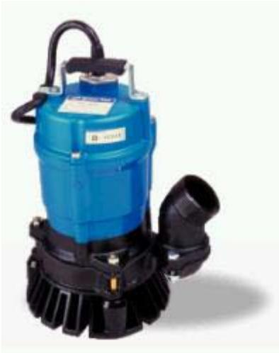
2", 53 GPM, 1/2 HP, 115V, Contractor grade submersible trash pump. Pumps sand, solids and debris with minimal wear and clogging. Optional float switch for automatic operation. \*\*\* [click here for more detailed info](#) \*\*\*
