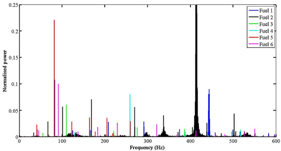
Figure 8: Normalised power spectrum at condition 4 for fuels 1-6
