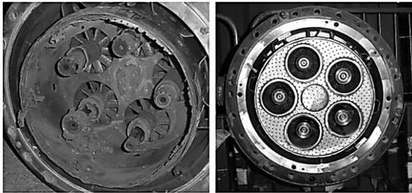
**Figure 1: Failed burner assembly [8]**
