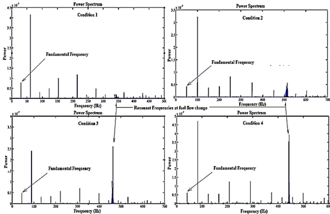
Figure 9: Power spectrum of vibration amplitude of combustor rig for fuel 1
