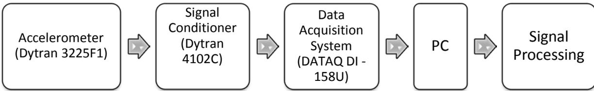
**Figure 4: Signal Acquisition**
