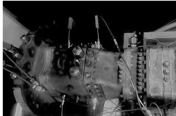
**Figure 3: Installed Vibration analysers on the rig**
