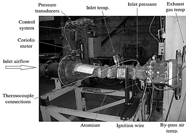
**Figure 2: Spey rig showing installed sensors on the rig**
