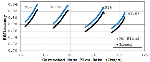
**Figure 1 (b): Bleed Impact on Compressor Performance Characteristics: Efficiency vs. Corrected Mass Flow**
