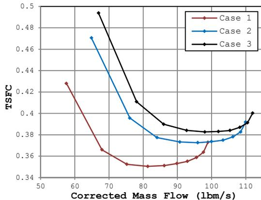
**Figure 5: Engine Cycle Impact Due to Varying Bleed Flow Extraction**
