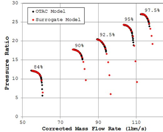
**Figure 3: Comparison between Surrogate and OTAC Compressor Model**
