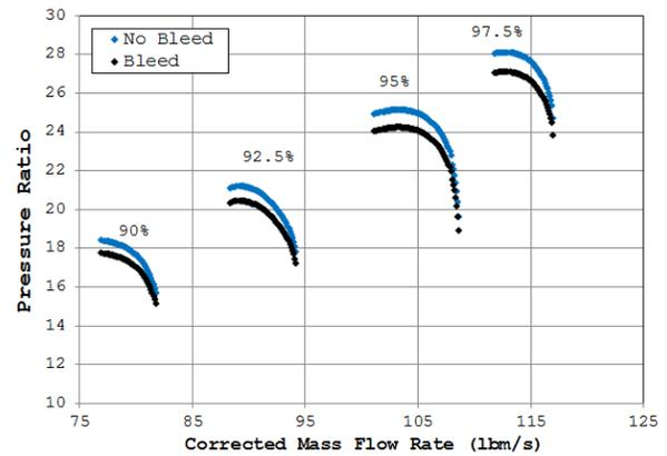
**Figure 1 (a): Bleed Impact on Compressor Performance Characteristics: Pressure Ratio vs. Corrected Mass Flow**
