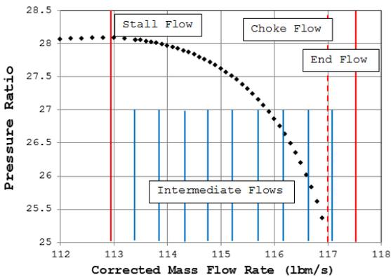
**Figure 2: Operating Flow Range Bracketing**
