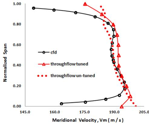
Figure 8 Vital Compressor Meridional Velocity
