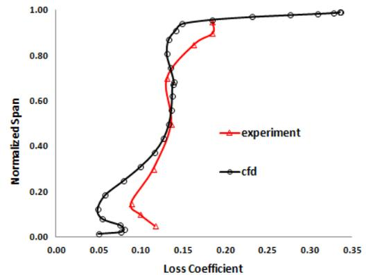
**Figure 3 Stage 35 Rotor Loss Coefficient**
