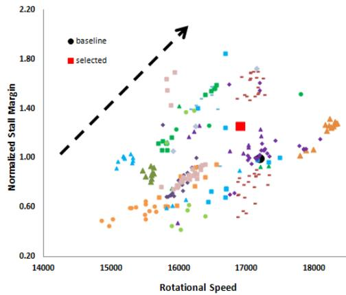
**Figure 14 Effect of Rotational Speed on Stall Margin**
