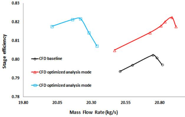
**Figure 19 Performance Map, Mass Flow - Efficiency**
