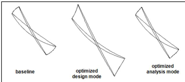
**Figure 15 Rotor Blade Comparisons**
