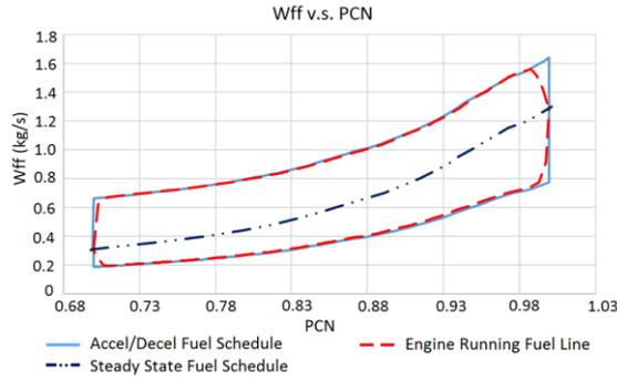
**Figure 20: Model Engine Wff v.s. PCN at Altitude = 1000m, Mach = 0.5**
