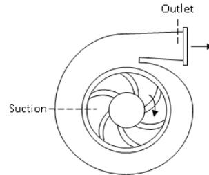
Figure 7: Schematic of Centrifugal Pump
