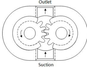
Figure 8: Schematic of Gear Pump
