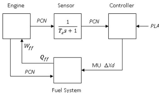
**Figure 15: Schematic of Integrated Engine, Control and Fuel System**
