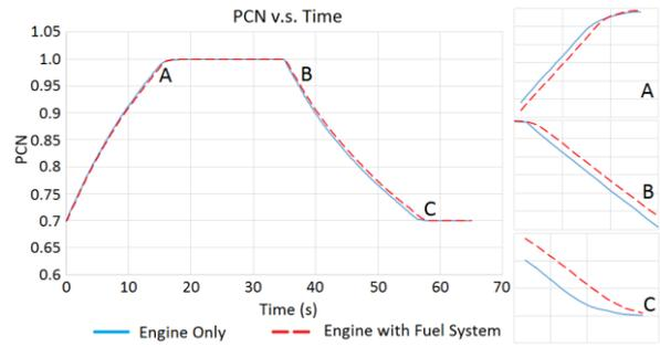
**Figure 22: Engine Relative Rotational Speed PCN Comparison for Engine with/without Fuel System**
