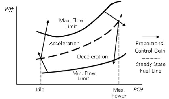
Figure 2: Fuel Schedule of Model Engine
