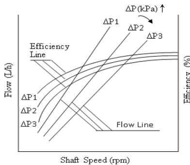
Figure 10: Typical Gear Pump Characteristic Map
