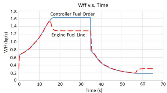
Figure 19: Model Engine Wff v.s. Time at Altitude = 1000m, Mach = 0.5
