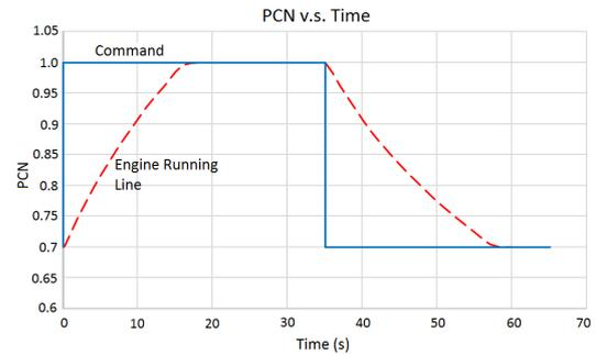
Figure 18: Model Engine PCN v.s. Time at Altitude = 1000m, Mach = 0.5
