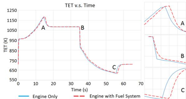
**Figure 23: Turbine Inlet Temperature TET Comparison for Engine with and without Fuel System**
