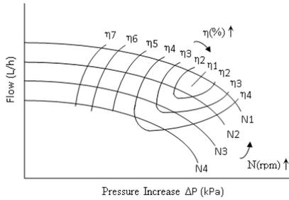
Figure 9: Typical Centrifugal Pump Characteristic Map
