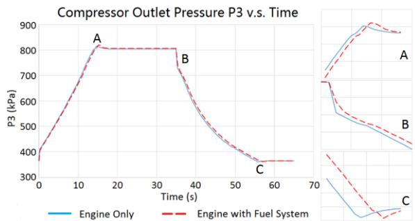
**Figure 24: Compressor Outlet Pressure  $P_3$  Comparison for Engine with and without Fuel System**
