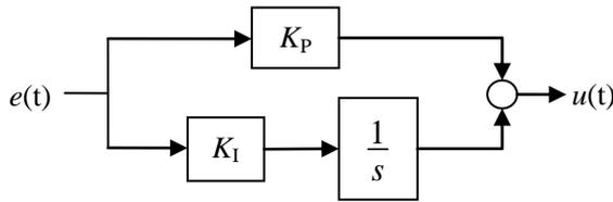
Figure 4: PI Controller Algorithm Diagram
