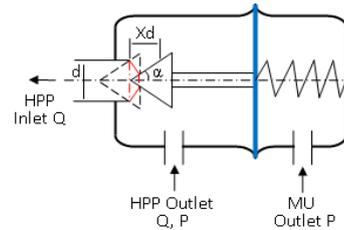
Figure 11: Schematic of constant pressure differential valve (CPDV)
