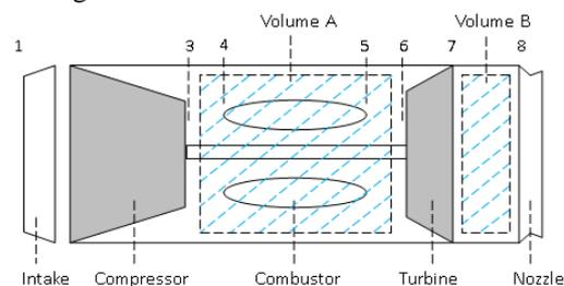
**Figure 1: Schematic of Single-Spool Turbojet Model Engine Configuration**
