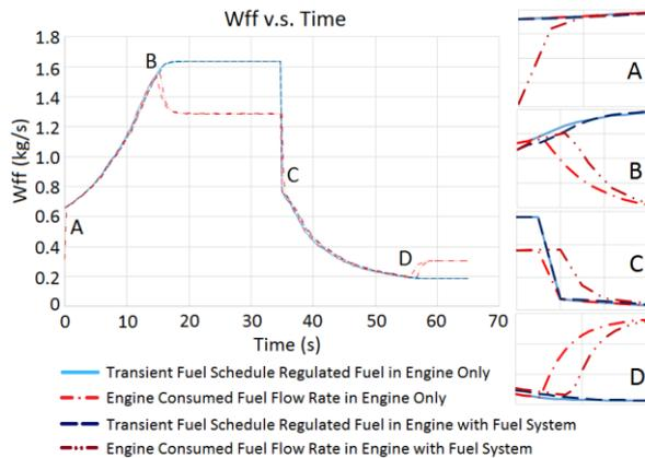
**Figure 21: Transient Fuel Schedules Comparison of Engine with and without Fuel System**
