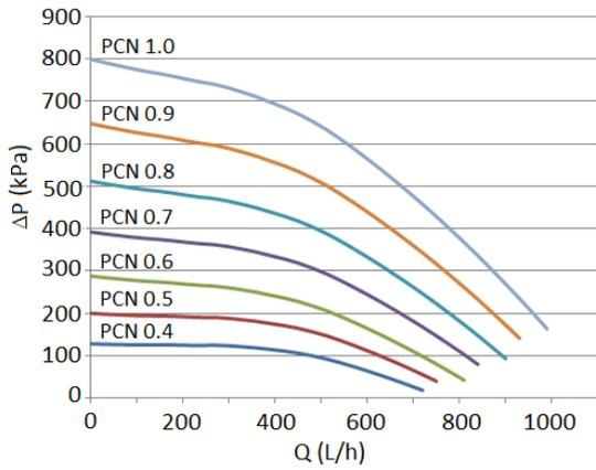
Figure 16: Characteristic Map of Centrifugal Pump
