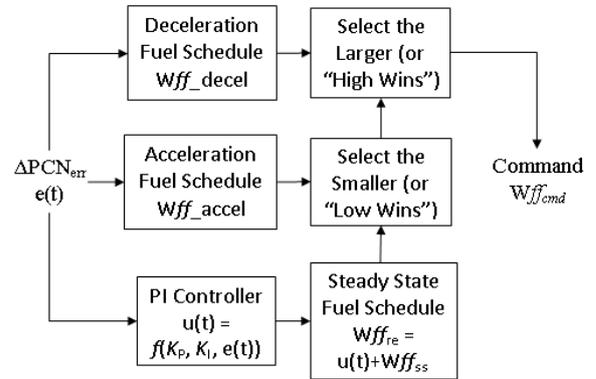
Figure 3: Diagram of Coupled Engine Controller and Fuel Selection Logic
