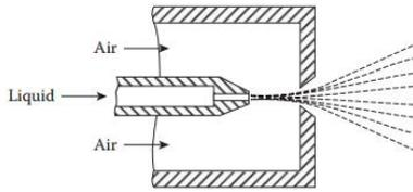
**Figure 13: Schematic of Fuel Injector [29]**
