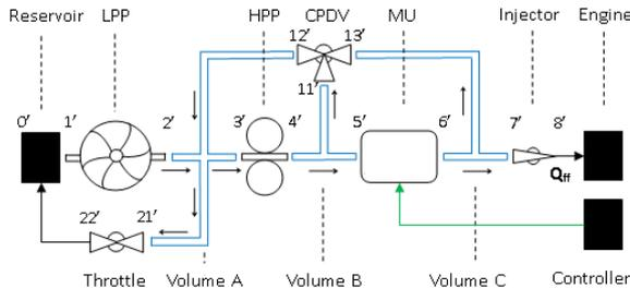
Figure 5: Schematic of Engine Fuel System
