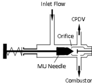
**Figure 12: Schematic of metering unit valve**
