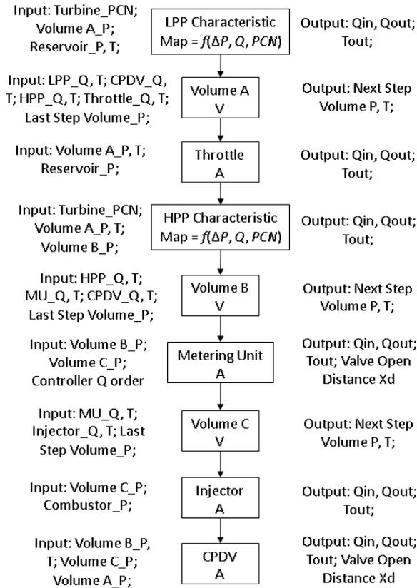
**Figure 14: Flow Chart of Fuel System Model**
