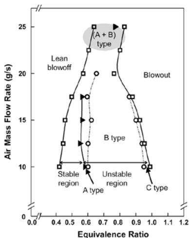
**Figure 2. The stability map for various inlet conditions**
