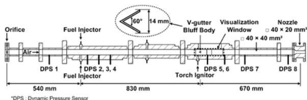
**Figure 1. Schematic of the ducted combustor with the bluff body**
