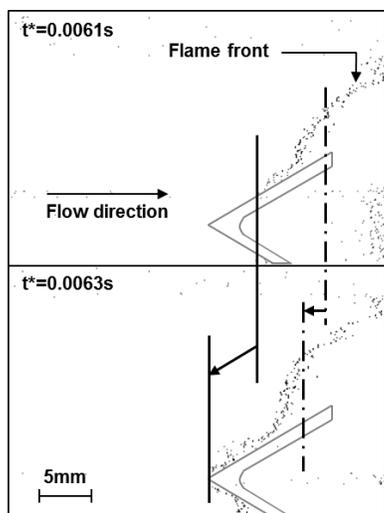
**Figure 6. The post-processing OH\* chemiluminescence images in the event of the flashback case**
