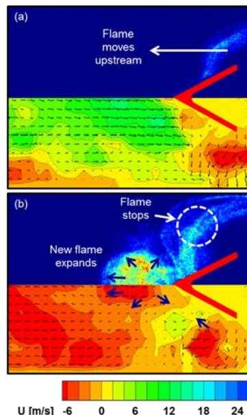
**Figure 5. The combination images of the instantaneous PIV and OH radical chemiluminescence at (a) the 101° phase of instability cycle, (b) the 130° phase of instability cycle**
