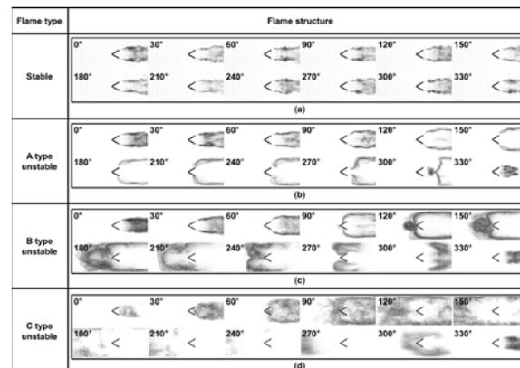
**Figure 3. The OH\* chemiluminescence images of the stable and unstable flames near the bluff body during one period**
