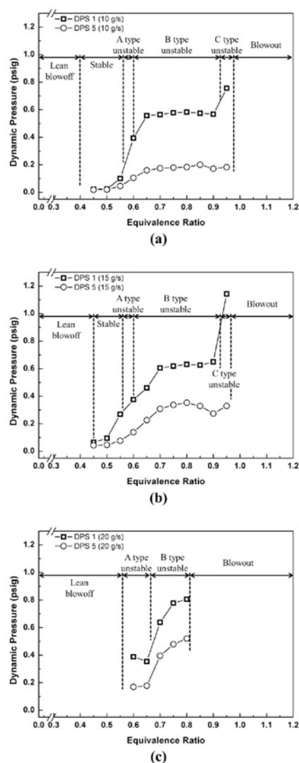
**Figure 4. The magnitude of the dynamic pressure with equivalence ratio at (a)  $m_a = 10$  g/s, (b)  $m_a = 15$  g/s, (c)  $m_a = 20$  g/s**
