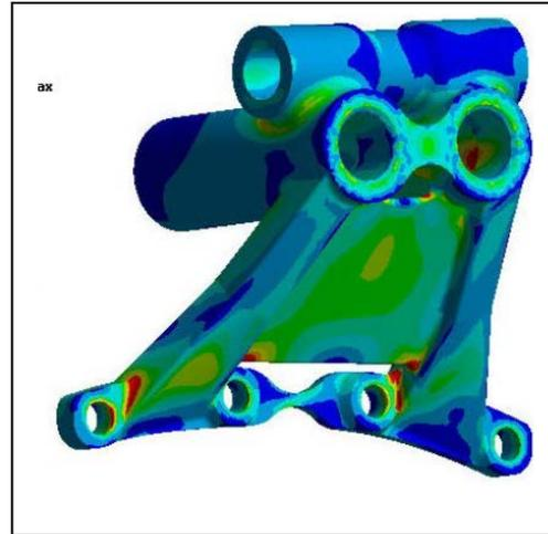
Figure 7: ANSYS analysis of re-designed TPE331 Engine Mount confirming design loads sufficient. Weight reduction of 56% from current design.
