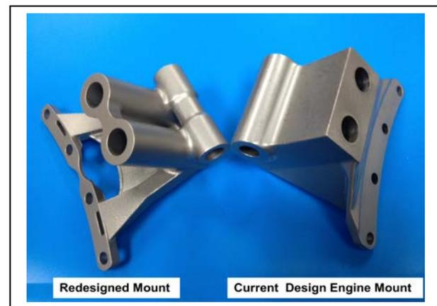
Figure 8: Photo of AM-built TPE331 Engine Mount next to current design TPE331 Engine Mount.
