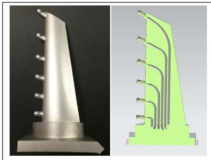
Figure 5: AM-built Inlet Booster Rake and cross-section.
