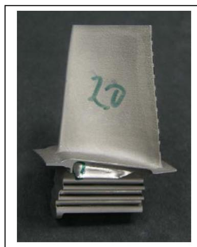
Figure 2: 2<sup>nd</sup> Stage HPT Blade for HTF7000
