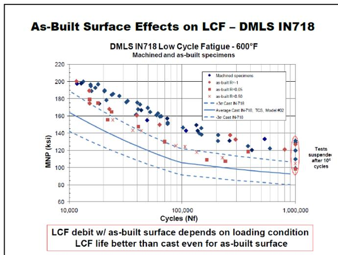
Figure 6: Surface Effects on LCF for DMLS 718
