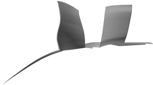
Fig. 2 Side View of 5deg. Swept Stator Model
