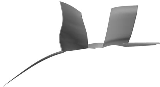
Fig. 3 Side View of 10deg. Swept Stator Model
