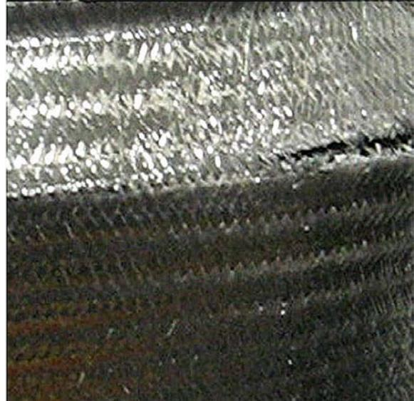
Figure 11. The braid reinforcement is highly resistant to crack growth due to the integrated multi-axial architecture.
