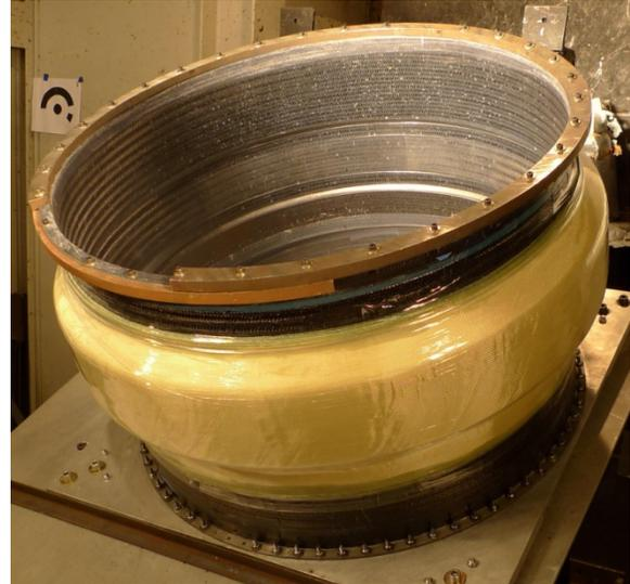
Figure 3. Braided composite fan case with aramid outer wrapping.
