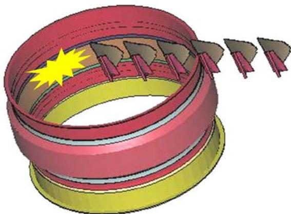
Figure 5. Fan blade flight path.
