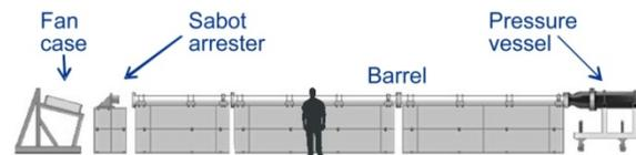
Figure 4. Schematic of the gas gun and the fan case mounted at an incline in front of the gun barrel.
