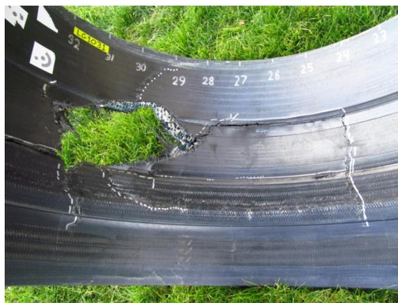
Figure 6. Damaged fan case after ballistic test.
