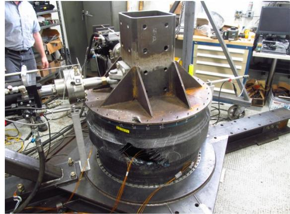
Figure 7. Ballistically-damaged fan case mounted on cyclic loading fixture.
