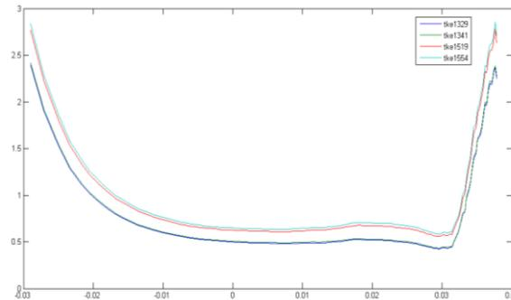
**Fig. 9.** Turbulent kinetic energy profile in the extrados of stator blade in the four cases: starting (1329 K), take-off (1554 K), cruise (1341K) and maximum cruise (1519)
