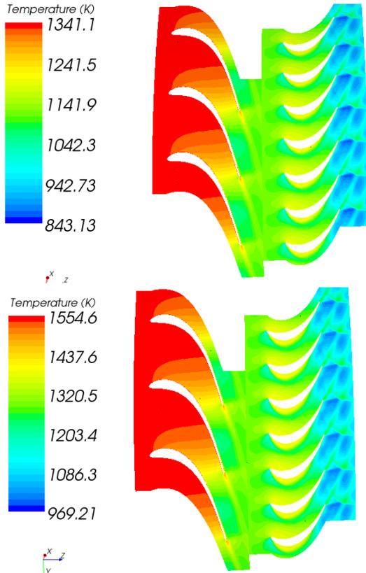
**Fig. 6.** Evolution of static temperature in two cases of initial temperatures: cruise (1341K) and take - off (1554 K)
