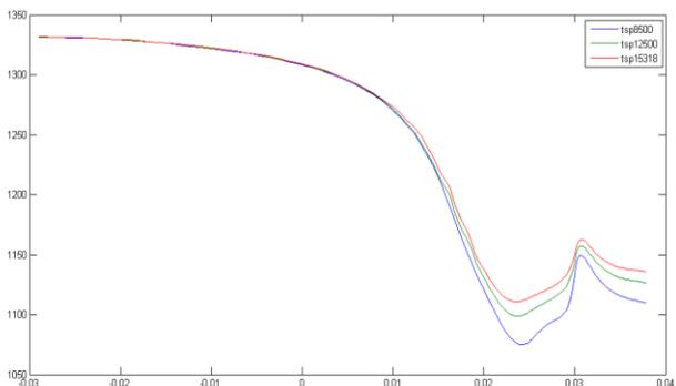
**Fig. 10** Temperature profile in the extrados of stator blade in three cases of rotor speed: 8500 tr/min, 12500 tr/min and 15183 tr/min (maximum operating speed)
