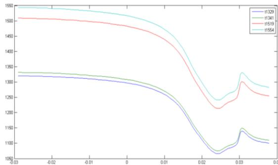
**Fig. 7.** Temperature profile in the extrados of stator blade in the four cases: starting (1329 K), take-off (1554 K), cruise (1341K) and maximum cruise (1519)
