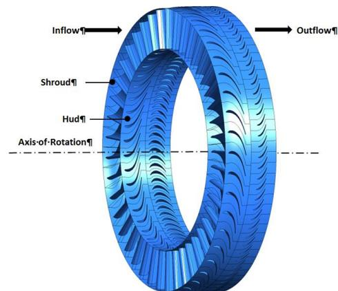
**Fig. 2.** The complete structure of the HPT
