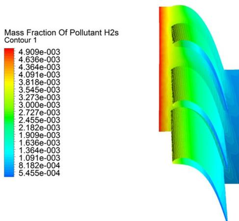
Fig. 16. Contour of the mass fraction of  $H_2S$  in the HPT
