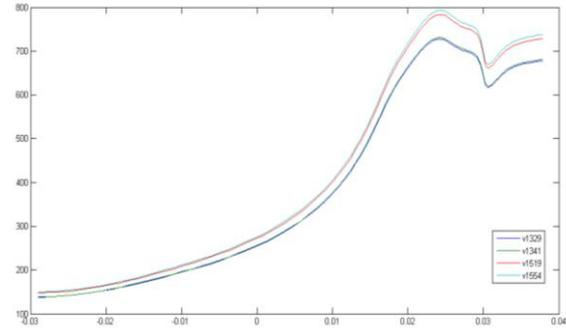
**Fig. 8.** Velocity profile in the extrados of stator blade in the four cases: starting (1329 K), take-off (1554 K), cruise (1341K) and maximum cruise (1519)
