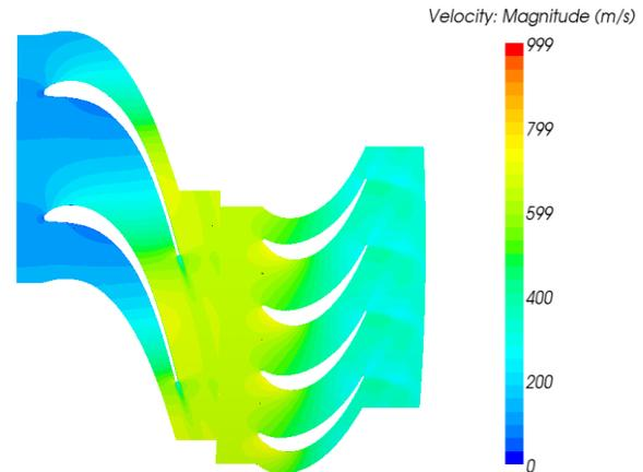
**Fig. 5.** Evolution of velocity in the HPT
