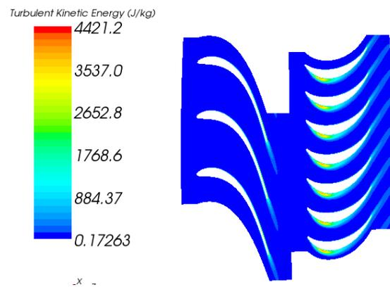
**Fig. 12** Turbulent kinetic energy evolution in the HPT in two cases of rotor speed: 8500 tr/min and 15183 tr/min (maximum operating speed)
