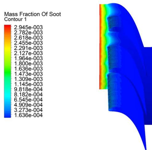
Fig. 18. Contour of the mass fraction of the soot in the HPT
