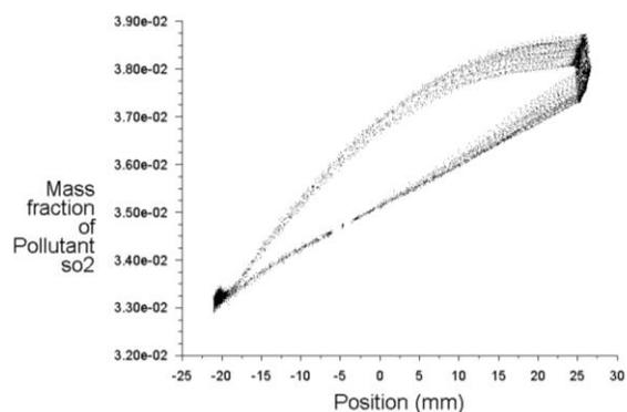
**Fig. 15.** Contour of the mass fraction of  $\text{SO}_x$  ( $\text{SO}_2$ ) among the axe z (the direction of flow) of the stator blade in the HPT
