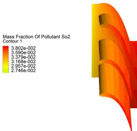
**Fig. 14.** Contour of the mass fraction of  $\text{SO}_x$  ( $\text{SO}_2$ ) in the HPT
