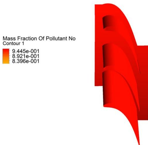
**Fig. 13.** Contour of the mass fraction of the  $\text{NO}_x$  (dominated by NO) in the HPT
