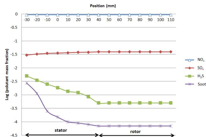
Fig. 19. Graphic of the pollutant mass fraction of the NO<sub>x</sub>, SO<sub>x</sub>, H<sub>2</sub>S et soot according the positions in the HPT
