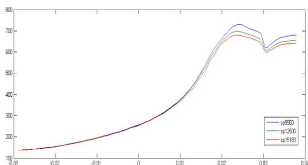
**Fig. 11** Velocity profile in the extrados of stator blade in three cases of rotor speed: 8500 tr/min, 12500 tr/min and 15183 tr/min (maximum operating speed)
