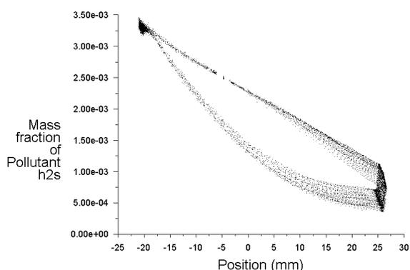
Fig. 17. Contour of the mass fraction of  $H_2S$  among the  $z$  (the direction of flow) of the stator blade in the HPT
