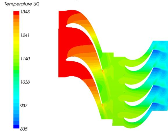
**Fig. 3.** Evolution of temperature in the HPT
