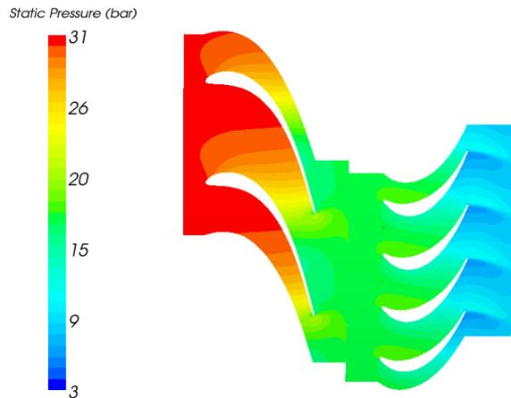
**Fig. 4.** Evolution of pressure in the HPT
