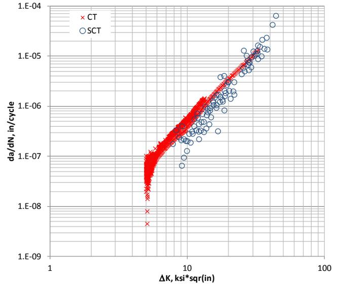
Figure 8. FCG results for large cracks generated using CT and SCT specimen geometry
