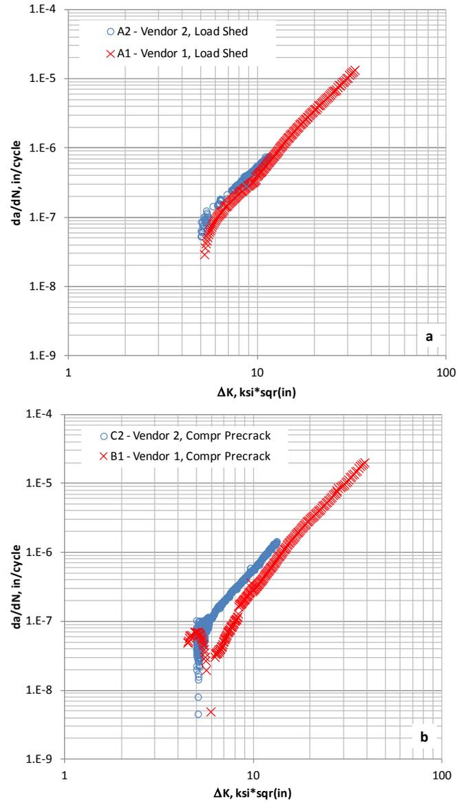
Figure 6. FCG curves for CT specimens tested by two different vendors at 600F and R=0.05 using ASTM load shedding (a) and compression pre-cracking (b) procedure
