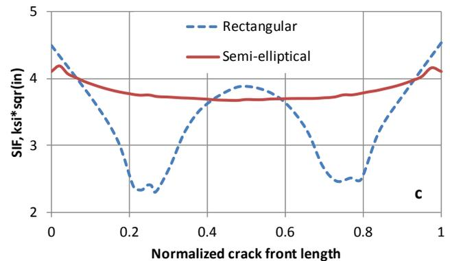
Figure 3. FIB notches of different shape (a, b) and corresponding stress intensities (c)
