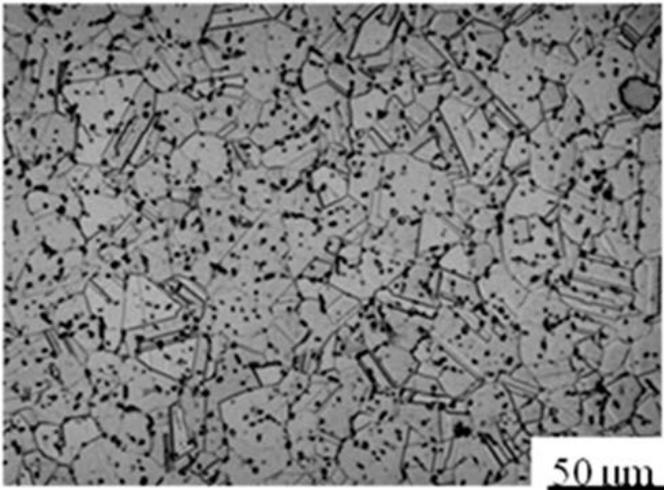
Figure 1. DP 718 microstructure
