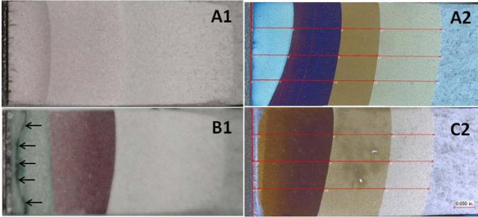
Figure 7. Fracture surfaces of CT specimens; FCG direction from left to right
