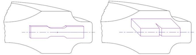
Figure 2. Orientation of the test specimens with respect to forging
