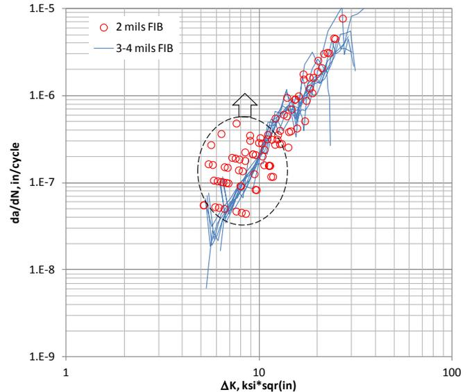
Figure 9. FCG results for small cracks generated using SCT specimen geometry with FIB notches
