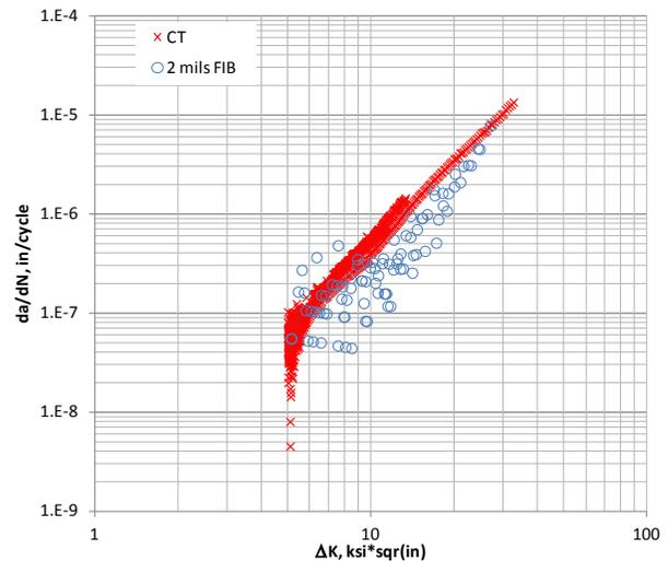
Figure 10. FCG results for small cracks generated using SCT specimen geometry with 2-mil FIB notches and large cracks generated using CT specimen geometry
