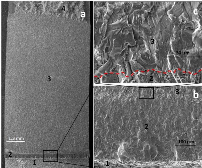
Figure 5. Overview (a) and microscopic details (b, c) of the compression pre-cracked CT specimen; 1- machined notch; 2- compression pre-crack; 3 – FCG growth under tension and 4 – final fracture
