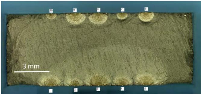
Figure 4. Fracture surface of SCT specimen with ten FIB notches
